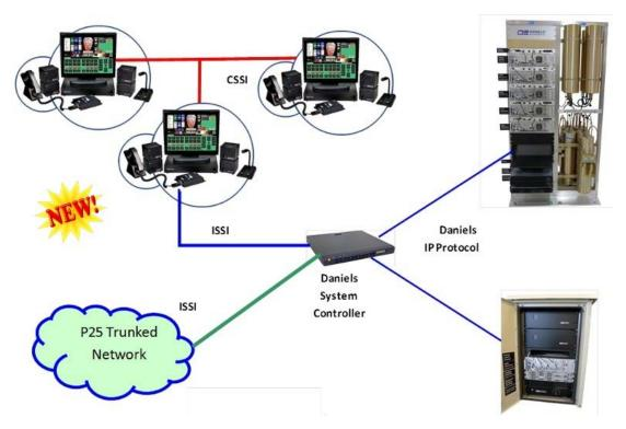
The Daniels P25 Trunked Radio System supports the Inter Sub-System Interface (ISSI) offering interconnectivity to other P25 trunked equipment:
